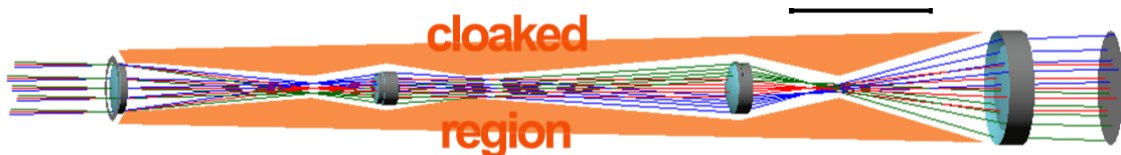
Figure 1: A ray diagram for a 4 lens cloaking device system.
