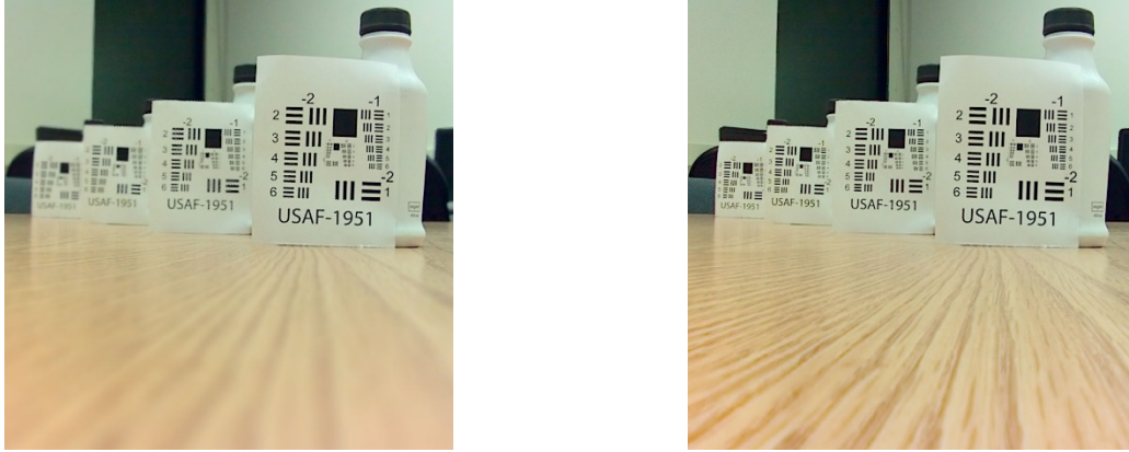
Figure A-3: Two 2D images generated with f/2.0 (left) and f/16.0 (right).
