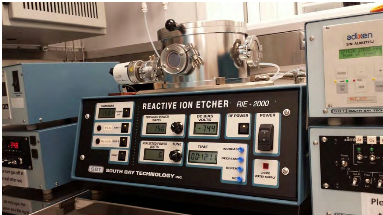
Figure 19: Image of the RIE setup in URNano cleanroom.
