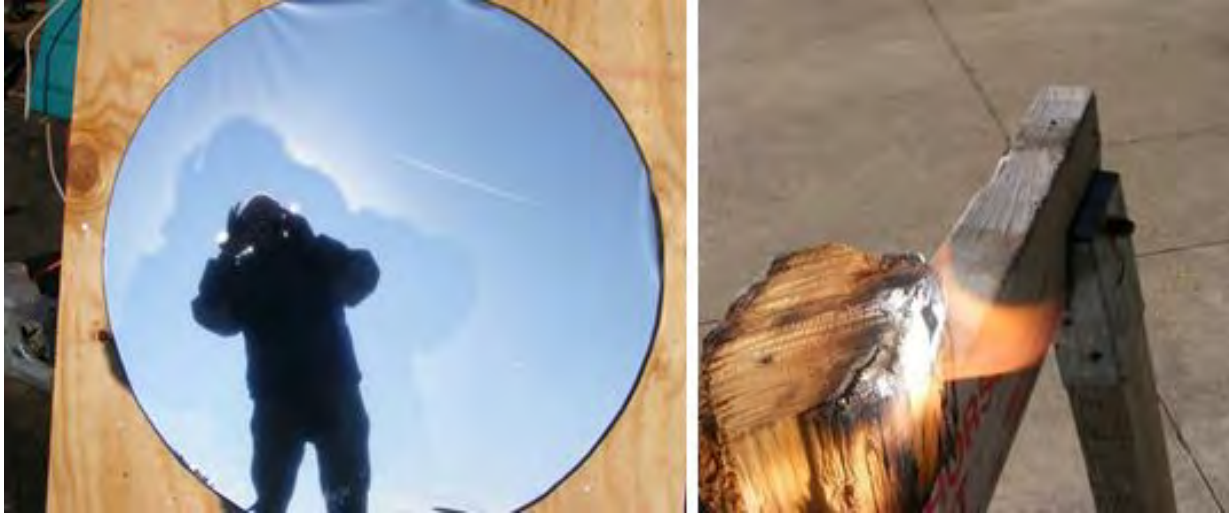
Figure 1: On left, Wayne Knox (our customer and competitor) takes a picture of his solar concentrator before a vacuum is applied. On right, the concentrator is able to ignite a block of wood.
