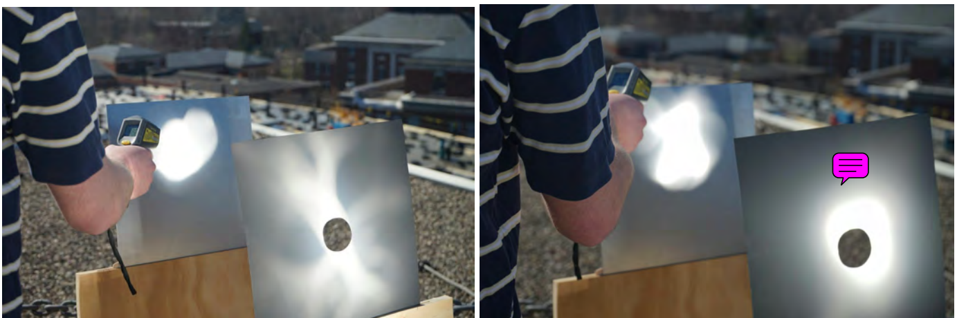
Figure 18: Left: Knox concentrator focused spot. Right: Senior Design concentrator focused spot. It can be noted that the Knox concentrator spot is extremely aberrated compared to the Senior Design concentrator spot.
