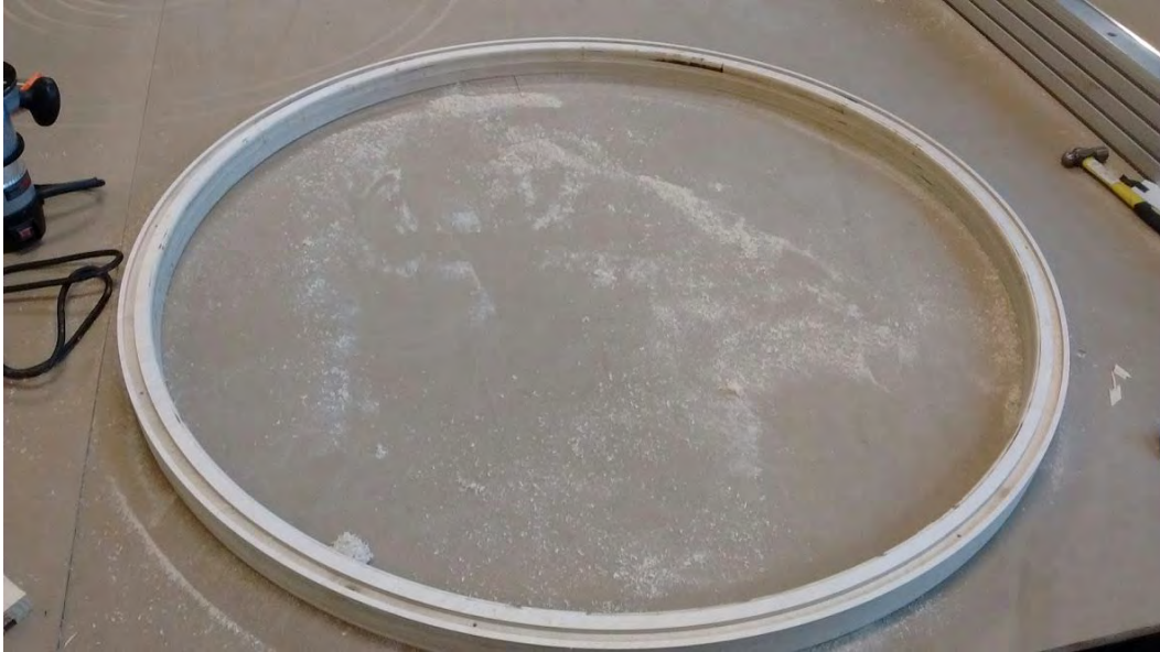
Figure 13: Bottom ring (47" OD, 44" ID, 2" depth) after manufacture on large CNC router and assembly with wood glue. This ring is comprised of two thinner rings, each of 1" depth. The rings are made of high-quality russian birch plywood.
