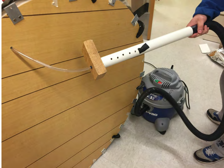
Figure 15: Adjustable pressure valve for controlling concentrator focal length
