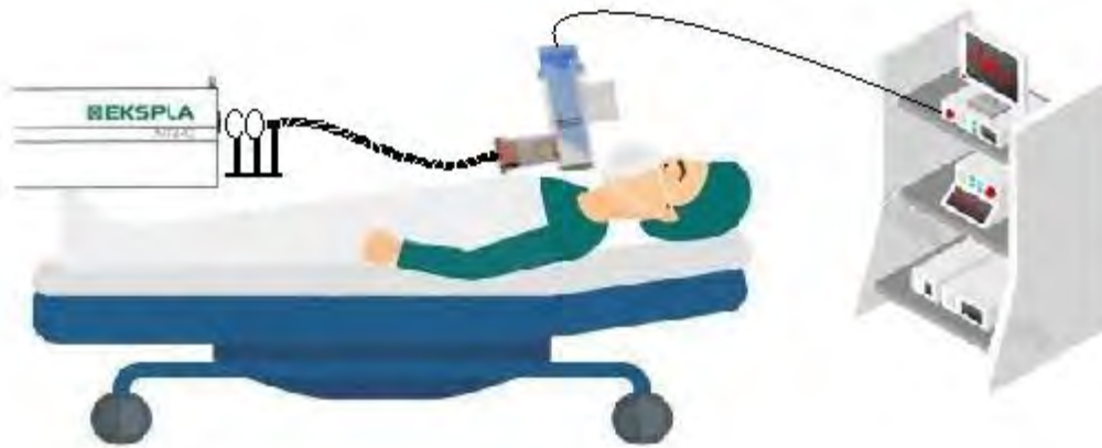
Diagram of Overall System: EKSPLA Nd:YAG pumped OPO laser, resizing optics, connecting lightguide, imaging probe, ultrasonic transducer, and accompanying computer system for recording images
