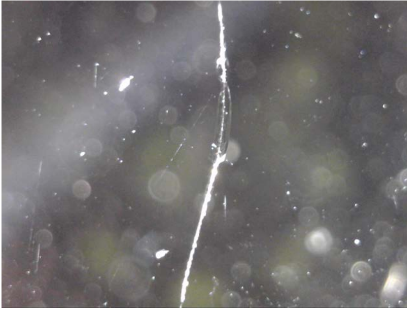
Figure 4: x20 mag picture of lens under Darkfield at 0 degrees. Ambient lighting still present.
