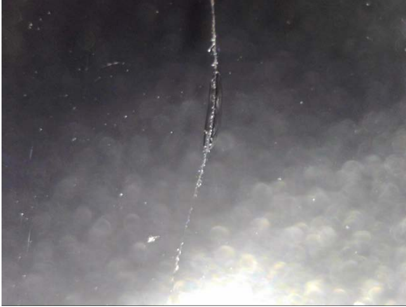
Figure 8: Picture of lens under darkfield lighting with source at 60 degrees from the ground. The light from the source can be seen at the bottom of the picture.
