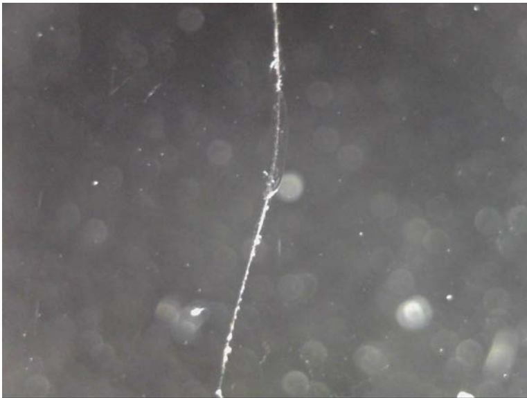
Figure 7: Picture of lens under darkfield lighting with source angled at 30 degrees above the ground. Less contrast of small features.
