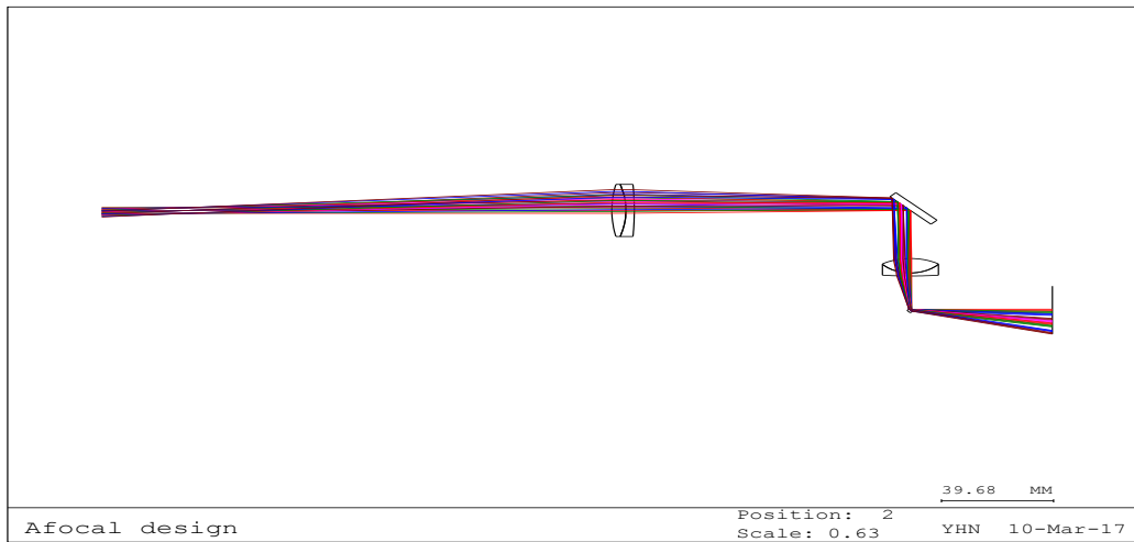
Figure 5: Afocal telescope assemble modeled into Code V. For performance, we verified RMS values throughout the scan field, each with a RMS WRE of 0.07 waves or less for a “diffraction limited” design using our wavelength and beam size.
