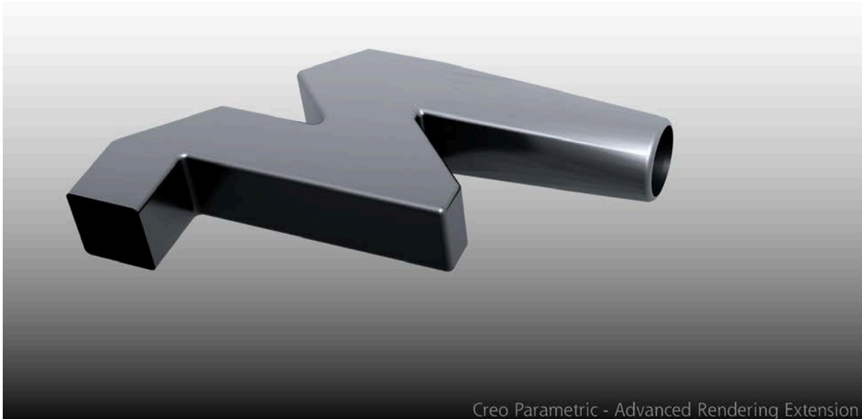
Figure 1: This is the preliminary exterior CAD model for a single eye, there will be two of these attached together to view both eyes. They will be attached in a way that the Inter-pupillary distance (IPD) is adjustable.
