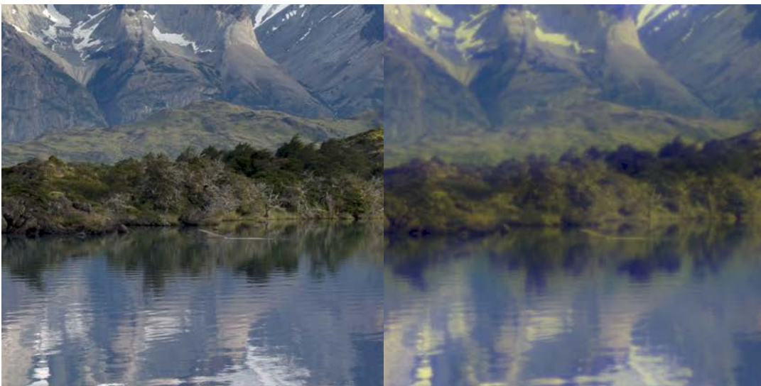
Figure 36: Zoomed in image simulation for 7 lens relay. Left image is the sample. Right image shows system results.
