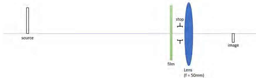
Figure 8. The single lens set up. In actual setup the film acts as a 45-degree horizontal mirror.
