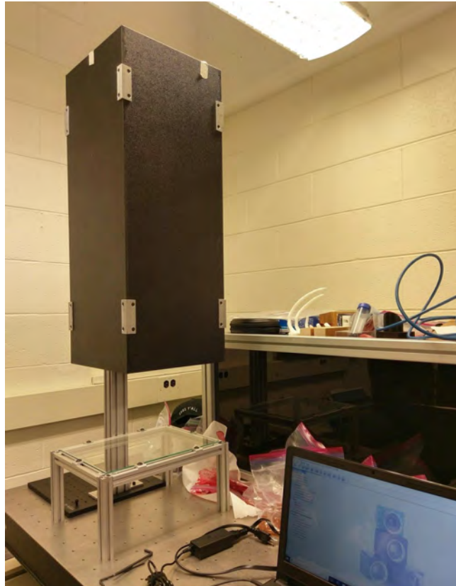
Figure 16: Current testing setup. The black box holds the light source, diffuser, and the fresnel lens. The height is adjustable.
