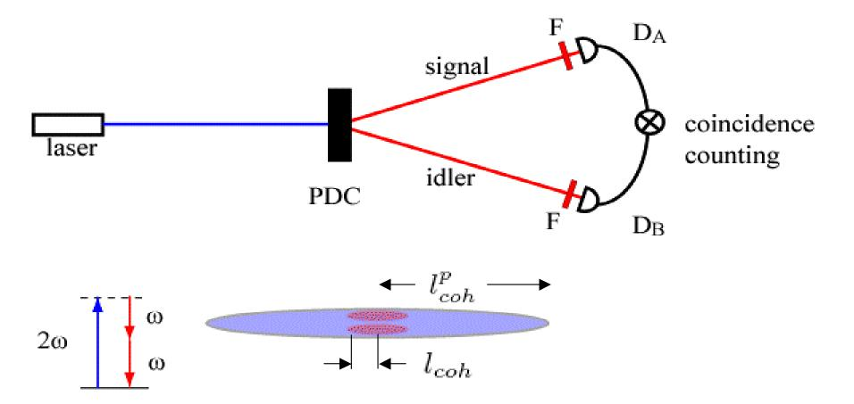
Length of two-photon wavepacket ~ coherence length of pump laser ~ 10 cm Coherence length of signal/idler photons ~  $c/\Delta\omega$  ~ 100 µm.
