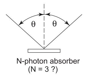
$\theta$  = 70 degrees write wavelength = 800 nm pulse energy = 130 µJ per beam pulse duration = 120 fs period =  $\lambda$  / (2 sin  $\theta$ ) = 425 nm
