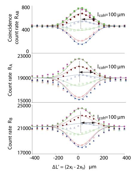
We see either a dip or a hump (depending on the value of  $\Delta L$ ) in both the single and coincidence count rates as we scan  $\Delta L'$ . Path-length difference is much larger than single-photon coherence length; this is not conventional (Young's) interference!
