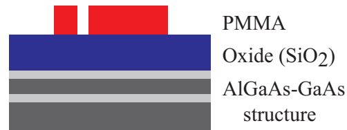
(4) Pattern inverse with e-beam & develop
