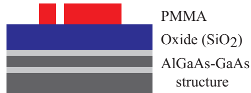
(4) Pattern inverse with e-beam & develop
