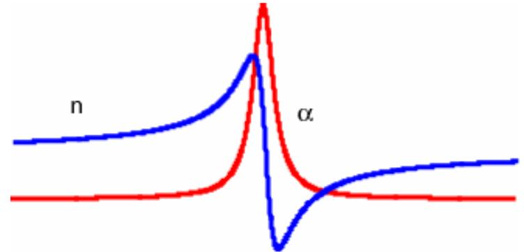
In a band-gap structure, material dispersion can be compensated by structural dispersion without inducing absorption
